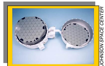
**Solar Collector Wafers** made of mostly silicon will be exposed to solar wind for two years.
